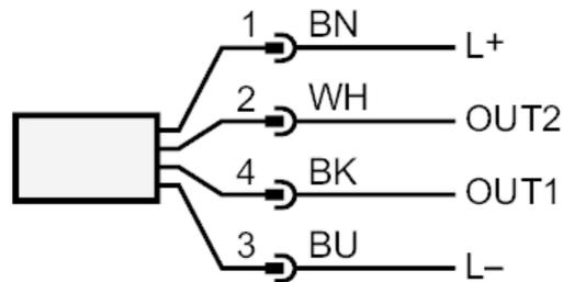
OUT1/IO-Link: switching output volumetric flow quantity monitoring
